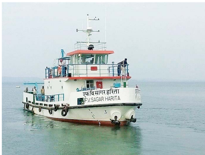
New generation fishing vessel FV Sagar Harita built by GSL, Goa for CIFT, Kochi
